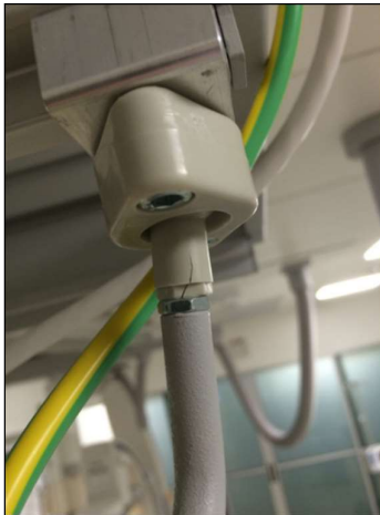
Arbore rulment din plastic rupt
